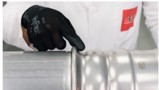
- Visual inspection of oversize pressing
