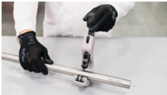
- Cutting the pipe to length
